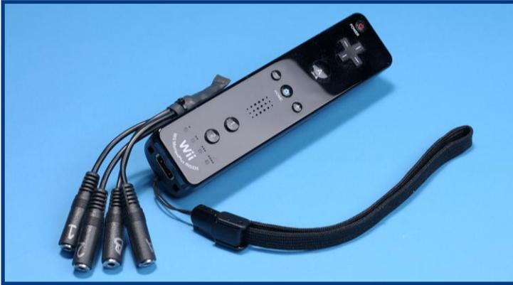
*This adapted Wiimote can be connected to a wide array of switches, readily available on the ability market; with the support of a qualified therapist, switches are chosen to accommodate a particular user's mobility – giving them access to a wide range of consumer gaming options*
